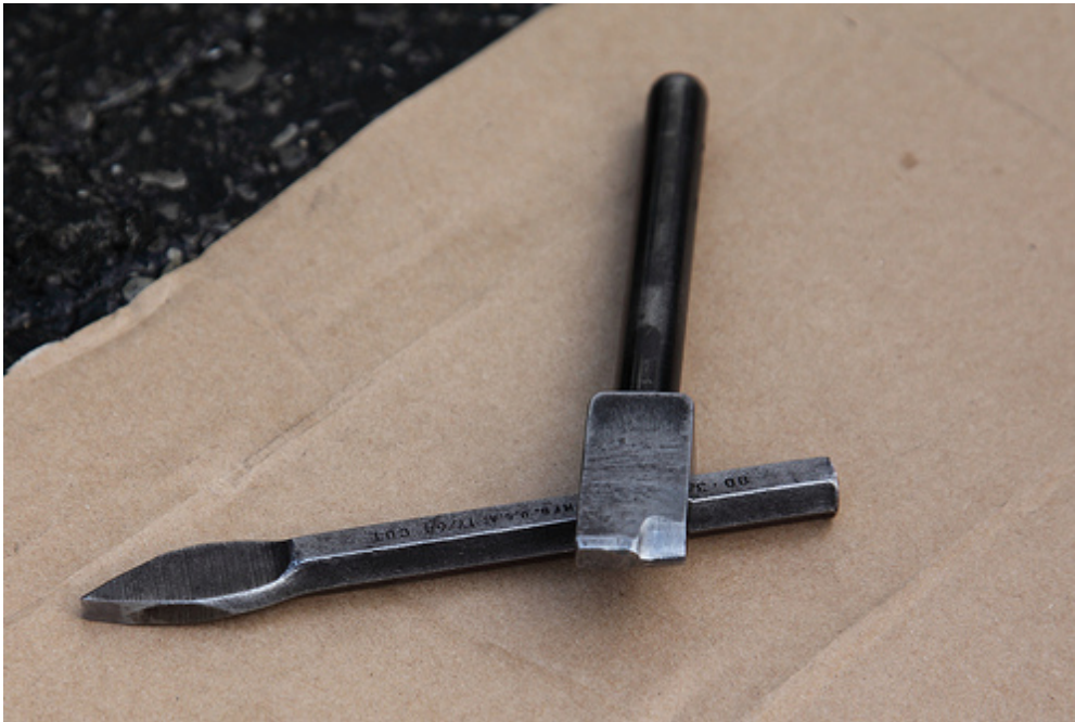
Staking tools, unstaking horizontal, skating vertical
