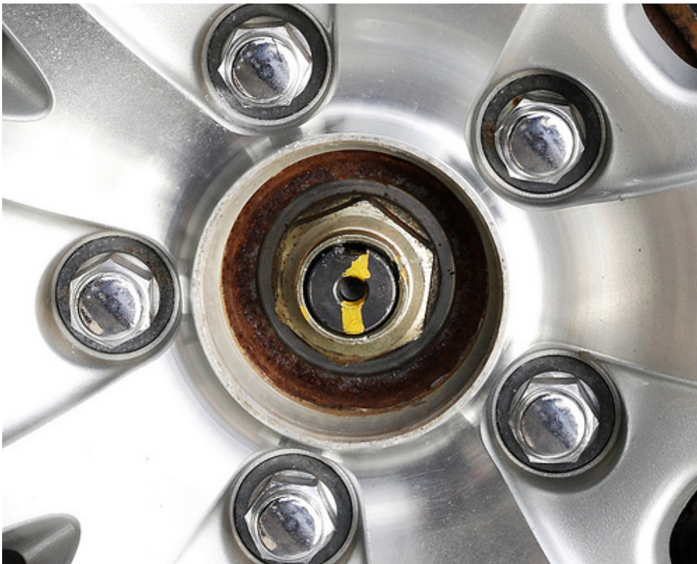
Axle nut in its final position.
