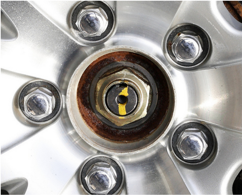
An axle nut re-installed at 180 ft-lbs. Notice that it's slightly past the original position.
