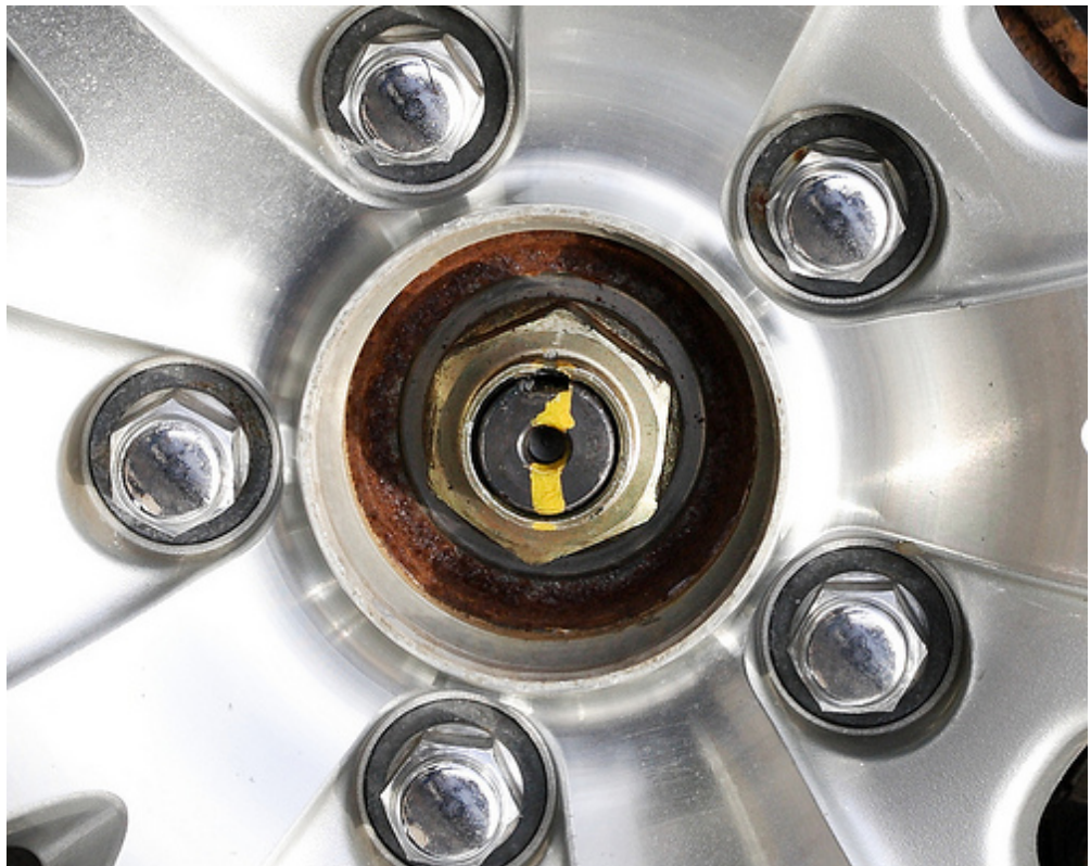
180 ft-lbs, estimated factory torque
