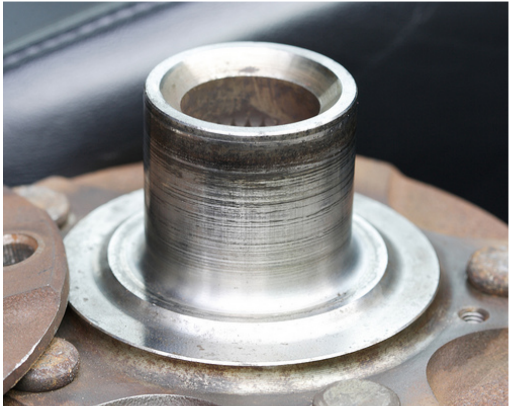
Good used rear hub (1.770" diameter)
