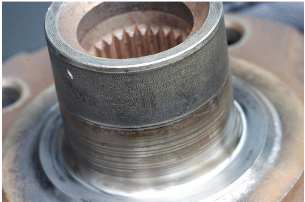
Damage used rear hub (1.763" diameter)
