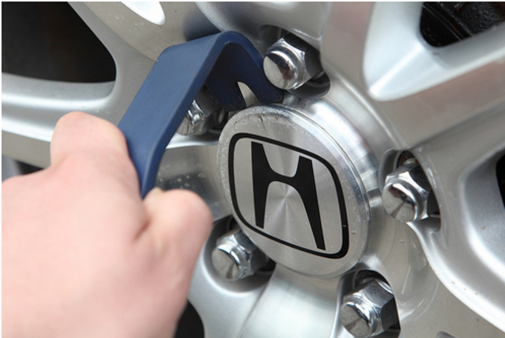
Center cap being removed.
