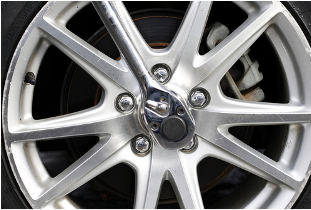
Ending position for final tightening.
